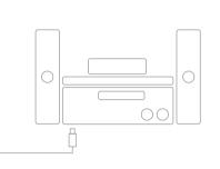
Connect an optical S/PDIF cable to the S/PDIF optical output of the A140 and the S/PDF optical input of an AV amplifier or home cinema system.
