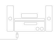
Connect an optical S/PDIF cable to the S/PDIF optical output of the A540 PVR and the S/PDF optical input of an AV amplifier or home cinema system.
