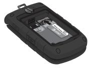
3. To remove the SIM, gently slide it out of the socket.
