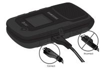
Note: The previous illustration is the correct and incorrect method for connecting the charger. If the incorrect method is attempted, damage to the accessory port will occur therefore voiding the phone's warranty.
