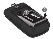
3. With the battery in position on the phone, place the cover back on the handset (1) then press down firmly (2). Press down along the edges to make sure the cover is flush with the phone and that there is a tight seal. 4. Turn the grooved dial clockwise until the cover locks.
