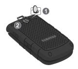
Use the grooves at the top of the cover to lift the cover up and away from the back of the phone (1).
