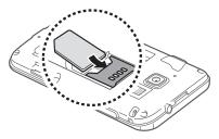
The antenna is located in the upper area on the back of the device. Do not remove the protective tape covering the antenna, as this can damage the antenna.
